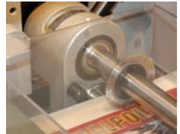
The slitting station can use either a shear (rotary), razor or crush knife.
