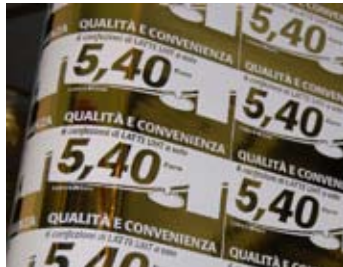
Digital presses cannot print gold-silver. Cold foil can apply the effects by glueing a metallic foil onto the web.
