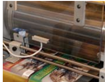
The semi-rotary die cutting unit accurately cuts the pre-printed web with a register system that reacts and compensates for misprints.
